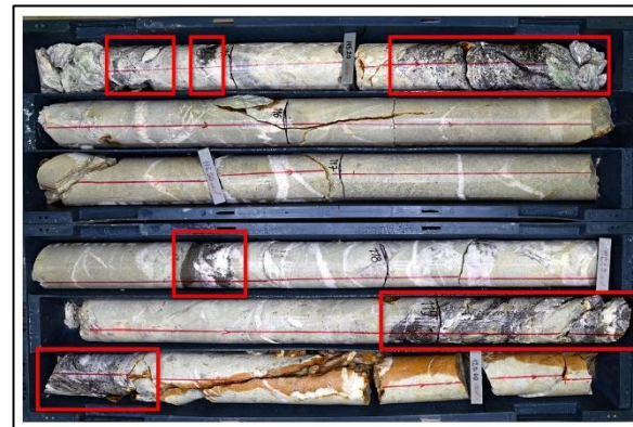
Figure: Gramusovici drillcore, showing phyllic/argillic alteration with sooty pyrite-chalcocite marked in red
