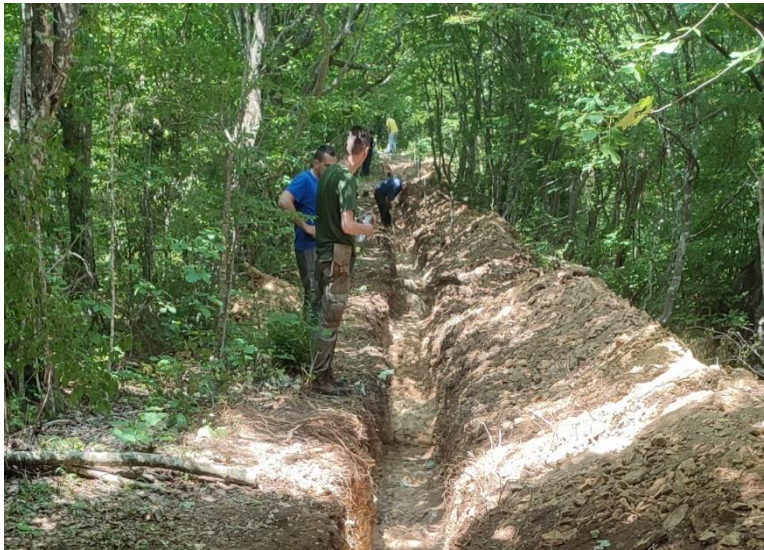
Figure: Channel sampling at Zekil along old forest track (note the shallow trench due to thin soil cover)
